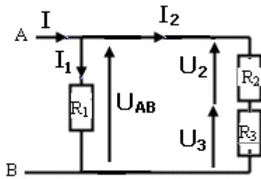
$$I_2 = \frac{U_{AB}}{R_2 + R_3} \quad \text{أي أن } U_{AB} = (R_2 + R_3)I_2$$
