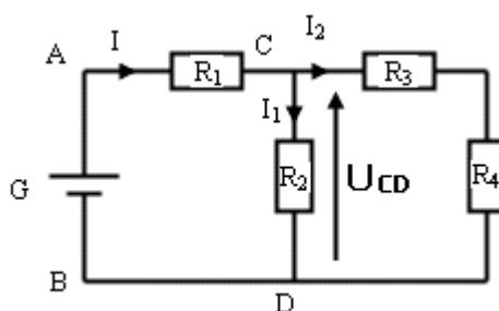
$$U_{CD} = R_2 I_1 \Rightarrow I_1 = \frac{U_{CD}}{R_2}$$
