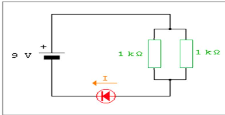
$$R_{eq} = \frac{R_1 \times R_2}{R_1 + R_2} = \frac{1\Omega \times 1\Omega}{1\Omega + 1\Omega} = 0,5k\Omega = 500\Omega$$
