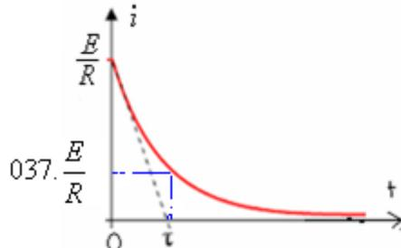
$$\begin{aligned} i &= \frac{dq}{dt} = \frac{d(C u_c)}{dt} = C \frac{du_c}{dt} \\ &= C \frac{d}{dt} \left[ E(1 - e^{-\frac{t}{\tau}}) \right] = C \left[ \frac{E}{\tau} \right] e^{-\frac{t}{\tau}} \\ &= C \frac{E}{R.C} e^{-\frac{t}{\tau}} = \frac{E}{R} e^{-\frac{t}{\tau}} \end{aligned}$$
