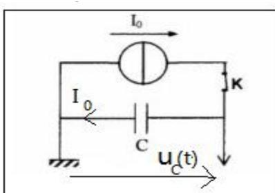
$$K = \frac{\Delta u_c}{\Delta t} = \frac{3V - 0}{5010^{-3}s - 0} = 60 Vs^{-1} \quad \text{المعامل الموجه : } u_c = Kt$$
