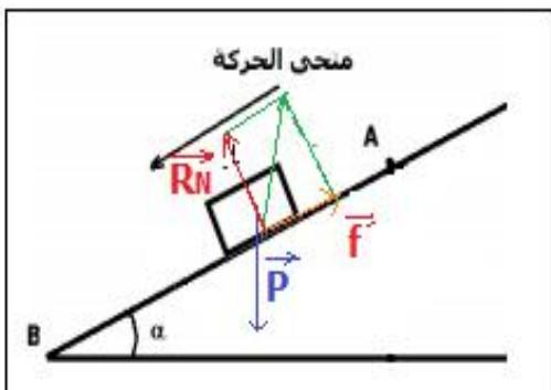
$$\Delta E_c = E_{cM} - E_{cB} = w(\vec{P})_{B \rightarrow M} + w(\vec{R})_{B \rightarrow M}$$
